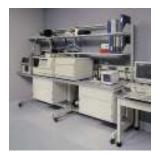
Strategies to build flexible, collaborative research environments include the use of casework systems that are easily moveable, limiting fixed elements in the laboratories, and containing hazards in the smallest workable area. Movable and height-adjustable laboratory benches with only minimal services are the norms in the interior of
