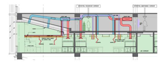
In addition to the initial demands, at least an additional 25% should be considered for future expansion. Space should be allowed in utility corridors, ceilings, and vertical chassis for future HVAC services, plumbing, and electrical needs. Service shutoff valves should be easily accessible, located in a box in the wall at the entry to the lab or in the ceiling at the entry. All pipes, valves, and clean-outs should be clearly labeled to identify the contents, pressure, and temperature.
